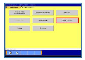
the valve body coding from the MDL beginning on page 8 (Learning Procedure - Valve Body or CVT Assembly Replacement) and upload to the ECU.
