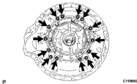
Fig. 637: Identifying Transmission Housing Bolts Courtesy of TOYOTA MOTOR SALES, U.S.A., INC.
