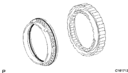
Fig. 451: Identifying O-Rings And No. 3 Brake Piston Courtesy of TOYOTA MOTOR SALES, U.S.A., INC.
