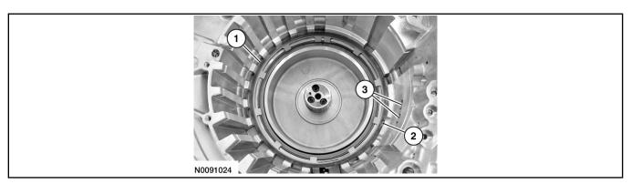
20. Install the 2-6 Piston Return Spring Compressor 307-633/2 on the transaxle case to center the intermediate (2, 6) clutch return spring.
