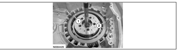
64. Using a suitable tool, seat the snap ring in the snap ring groove.
