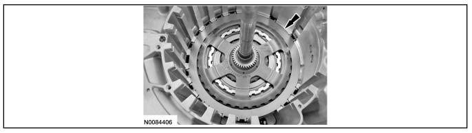
33. Install the Shim Selection Gauge 307-300 on the transaxle case.
