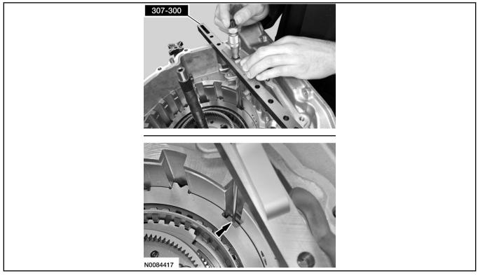
49. Using a suitable depth gauge, measure and record as measurement E, the distance from the top of Shim Selection Gauge 307-300 to the top of the low/reverse clutch at 3 different points and average the 3 distances.
