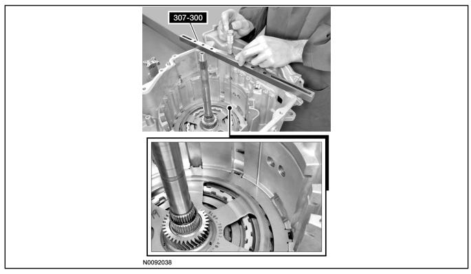
36. Subtract measurement B from measurement A The clearance should be between 0.240 mm (0.009 in) and 2.60 mm (0.102 in). If the clearance is out of range, check the intermediate (2, 6) clutch pack for correct installation. If the intermediate (2, 6) clutch pack is correctly installed, install a new clutch pack.
