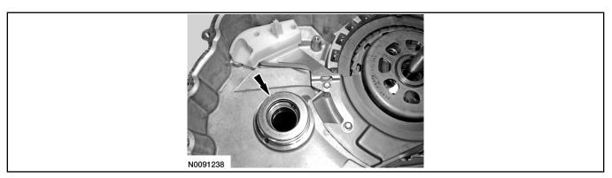
82. Simultaneously install the drive/driven sprocket and chain assembly. Lightly tap on the driven sprocket to be sure it is fully seated in the case.
