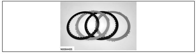
32. Install the intermediate (2, 6) clutch assembly, temporarily reversing the top friction and steel plates for the clutch stack-up measurement.
