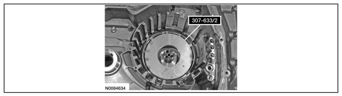
21. Install the 2-6 Piston Return Spring Compressor 307-633/1 on the snap ring.
