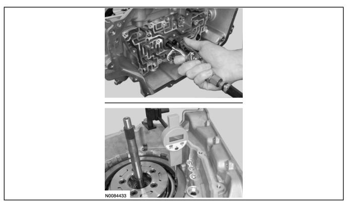
68. Install the front planetary sun gear and shell assembly.
