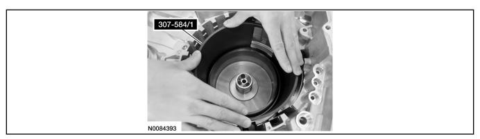
17. Remove Forward/Intermediate Spring Compressor 307-584/1 and Clutch Piston Seal Protector 307-632.
