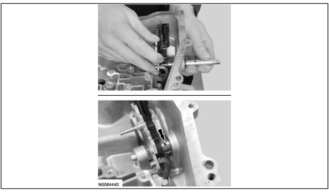
75. Install the manual control shaft roll pin.
