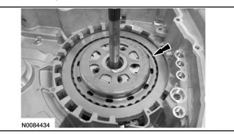
69. Install the No. 10 thrust bearing.
