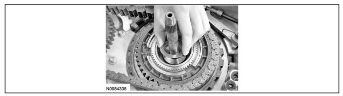
84. Install the No. 13 thrust washer.
