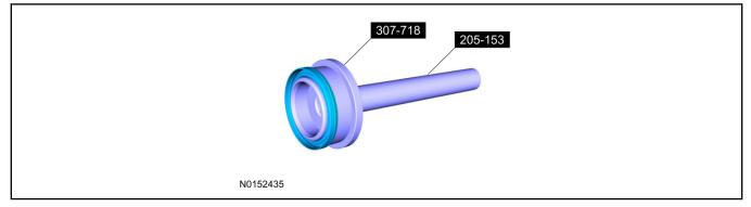
93. Using the Handle 205-153 and Axle Seal Installer 307-718, install the new RH halfshaft seal.
