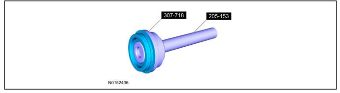
91. Using the Handle 205-153 and Axle Seal Installer 307-718, install the new RH halfshaft seal.
