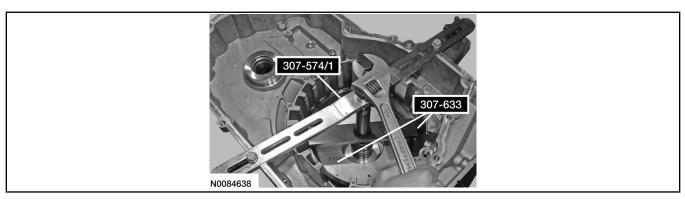
24. Remove the Forward Clutch Spring Compressor 307-574/1 and the 2-6 Piston Return Spring Compressor 307-633.
