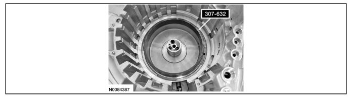
11. Lubricate the seals on the intermediate (2, 6) clutch piston with clean transmission fluid.
