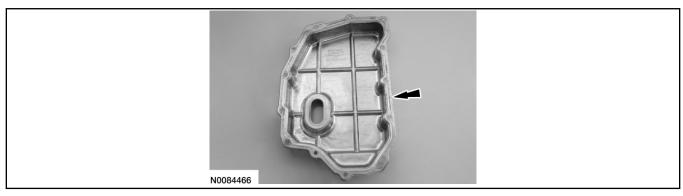
117. Apply silicone to the main control sealing surface of the transaxle case.
