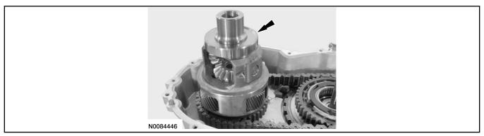
87. Install the No. 15 thrust bearing.
