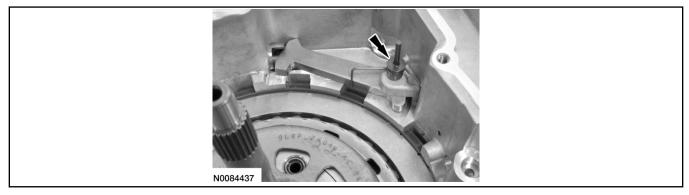
72. Install the park pawl actuator rod in the Transmission Range (TR) sensor.
