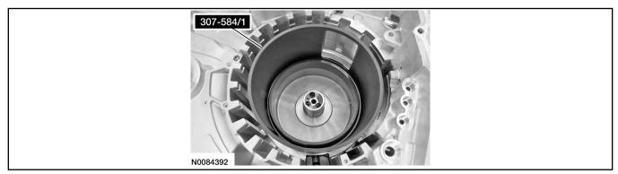
16. Using Forward/Intermediate Spring Compressor 307-584/1, push the intermediate (2, 6) clutch piston into the clutch cylinder by hand.
