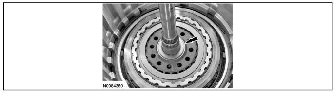
29. Install the direct/intermediate clutch hub and rear sun gear assembly.
