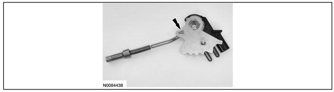
73. Position the park pawl aside and position the park pawl actuator rod and the TR sensor in the transaxle case.
