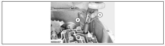
105. Install the bypass valve spring.
