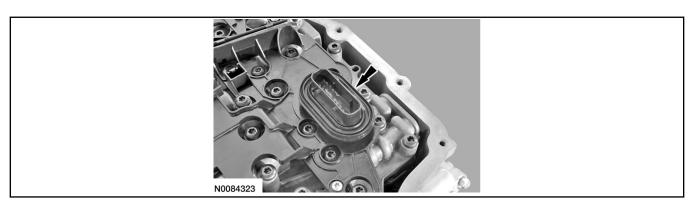
114. Connect the TR sensor electrical connector.
