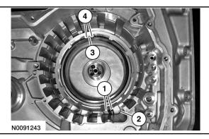
14. Remove the intermediate (2, 6) clutch piston return spring.
