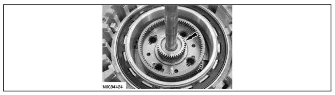
56. Install the center carrier/front ring gear assembly.
