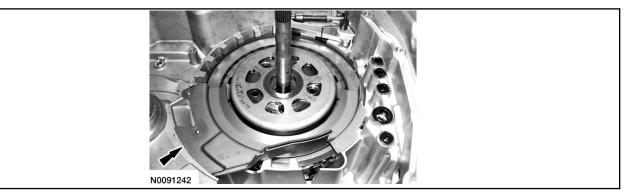
79. Install the lube funnel and position the alignment pin in the alignment hole.
