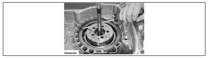
65. Install Dial Indicator Gauge With Holding Fixture 100-002 or a suitable dial indicator on the transaxle case and position the plunger on the top forward (1, 2, 3, 4) clutch friction plate.
