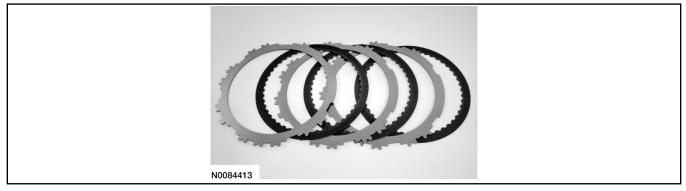
42. Align the low/reverse clutch pack with the pressure plate and install it in the transaxle case temporarily reversing the wave spring and top steel plate.
