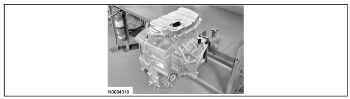
124. Remove the Holding Fixture 307-625.
