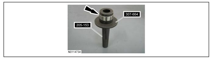
3. Using the Handle 205-153 and the Bushing Installer 307-664, install the new bushing in the transaxle case.
