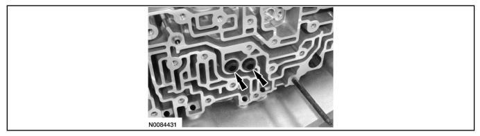
67. Apply 483 kPa (70 psi) of air pressure to the forward (1, 2, 3, 4) clutch piston port while recording the clutch pack clearance on the dial indicator. The clearance should be between 0.076 mm (0.002 in) and 1.840 mm (0.072 in). If the clearance is out of range, check the forward (1, 2, 3, 4) clutch pack for correct installation and the transaxle for correct assembly. If the forward (1, 2, 3, 4) clutch pack is correctly installed, install a new forward (1, 2, 3, 4) clutch pack.
