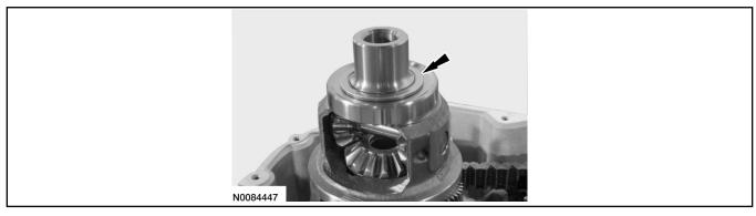
88. Install the Turbine Shaft Seal Protector 307-635 on the input shaft.
