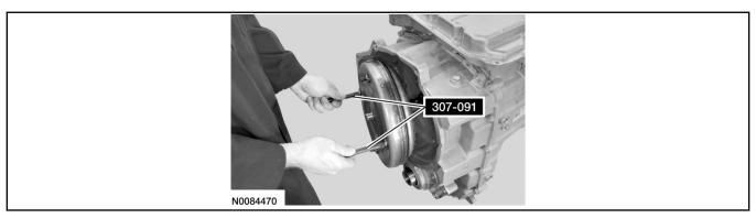
121. Remove the Torque Converter Handle 307-091.
