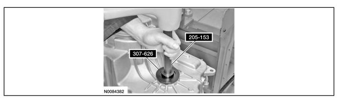
6. Install a new manual control shaft seal on Manual Lever Seal Installer 307-581.
