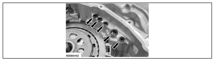
78. Position the transmission fluid baffle in place.
