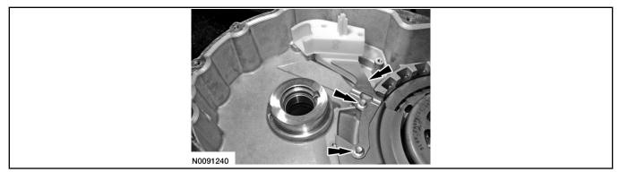
81. Install the No. 12 thrust bearing.
