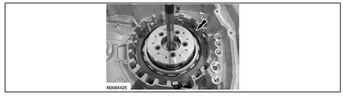
60. Soak the forward (1, 2, 3, 4) clutch pack in clean automatic transmission fluid.
