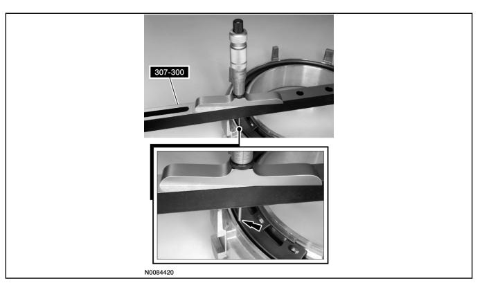
45. Using a suitable depth gauge, measure and record as measurement B, the distance from the top of Shim Selection Gauge 307-300 to the leg surface of the center support.
