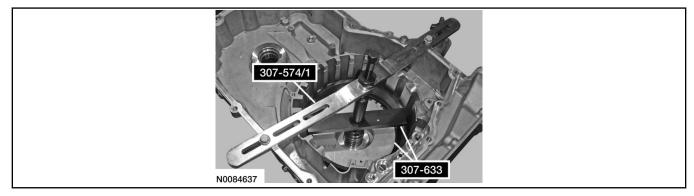
25. Install the intermediate (2, 6) clutch apply ring. Tap the ring in place using a suitable tool.
