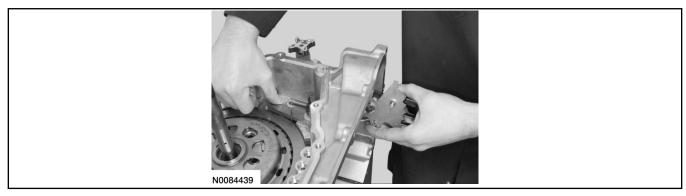
74. Install the manual control shaft and align the roll pin holes.
