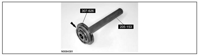
5. Using the Differential Seal Installer 307-626 and Handle 205-153, install the new LH halfshaft seal in the transaxle case.
