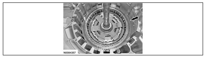
39. Install the rear planetary carrier/center ring gear assembly.
