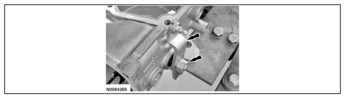
77. Install the 5 new clutch feed seals.
