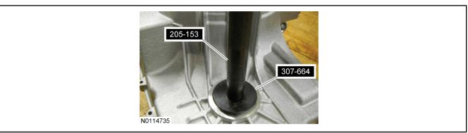
4. Assemble the Handle 205-153 and Seal Installer 307-626. Install a new LH halfshaft seal on the Differential Seal Installer 307-626.
