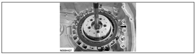
62. Install the forward (1, 2, 3, 4) clutch pressure plate.
