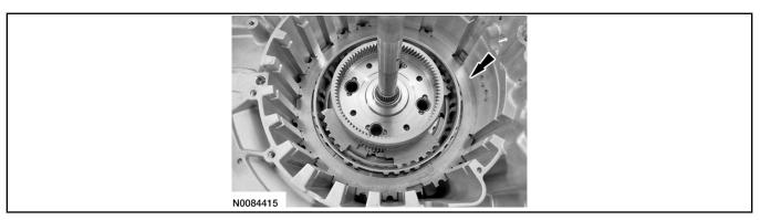
41. Soak the low/reverse clutch in clean automatic transmission fluid.
