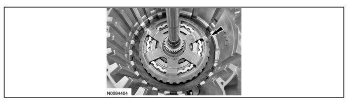
31. Soak the intermediate (2, 6) clutch assembly in clean transmission fluid.
