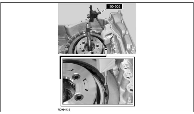
66. Install the new low/reverse and forward (1, 2, 3, 4) clutch feed seals in the transaxle case.
