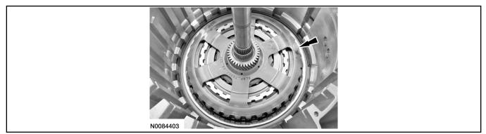
30. Install the intermediate (2, 6) wave spring assembly.
