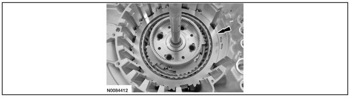
43. Install the Shim Selection Gauge 307-300 on the side of the center support with the long support legs.
