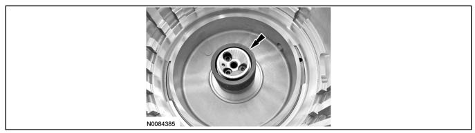
9. Remove Input Shaft Support Seal Installer 307-578/1.
