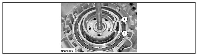
58. Install the front planetary/rear ring gear assembly.
