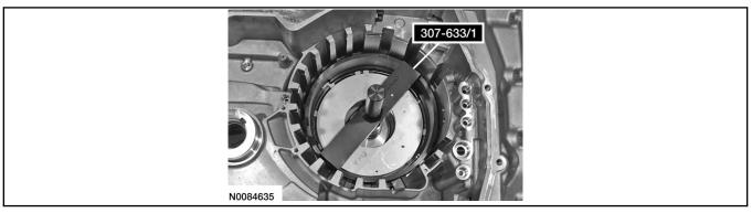
22. Install Forward Clutch Spring Compressor 307-574/1 on the transaxle case.
