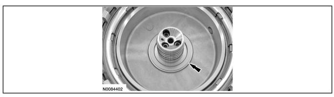
27. Install the overdrive/direct clutch assembly.
