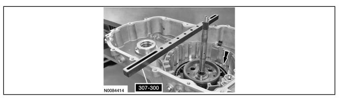
48. Using a suitable depth micrometer, measure and record as measurement D, the distance from the Shim Selection Gauge 307-300 to the top of the OWC.
