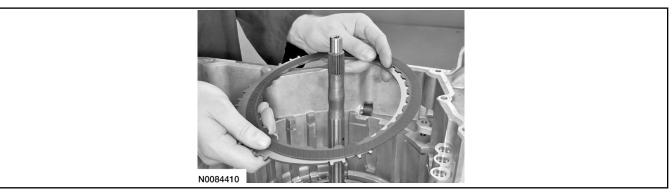
38. Install the One-Way Clutch (OWC) assembly.
