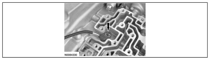
104. Assemble the bypass valve in the sleeve and install the assembly in the case.
