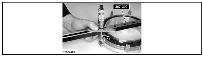
46. Subtract measurement B from measurement A and record as measurement C.
