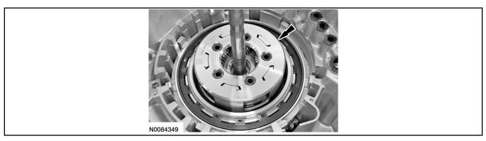
59. Install the forward (1, 2, 3, 4) clutch wave spring.
