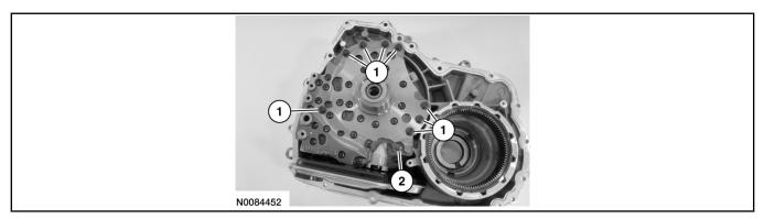
98. Install the transmission fluid baffle and the 2 bolts.
