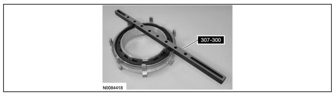
44. Using a suitable depth gauge, measure and record as measurement A, the distance from the top of Shim Selection Gauge 307-300 to the contact surface of the low/reverse clutch piston.
