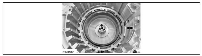
15. Install Forward/Intermediate Spring Compressor 307-584/1 on the intermediate (2, 6) clutch piston.
