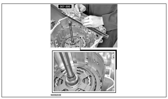
35. Using a suitable depth gauge, measure and record as measurement B, the distance from the top of Shim Selection Gauge 307-300 to the transaxle case step above the intermediate (2, 6) clutch.
