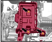
Remove securing clip in -direction of arrow-.
