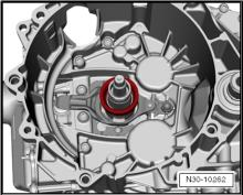
Small engagement bearing only fits in one position due to 4 grooves.
