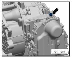
Attach all retainers and brackets to front of gearbox.
