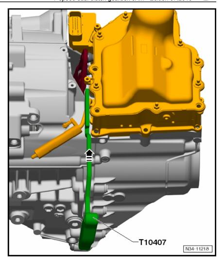
Far enough until groove lines up with housing rib -arrow-.
