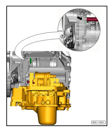
The "sticking" gear actuator -arrow- can be pressed by hand into its "removal position". To do this, push a selector fork behind the parking lock cover. How to do this is described in the following work procedure:
