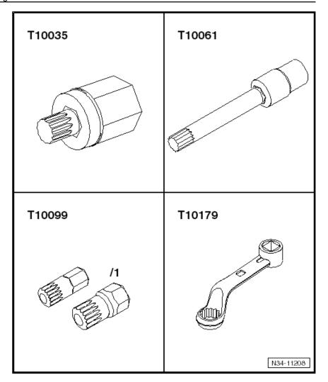
A bolt is located in the starter motor hole. Bit -T10061- can be used instead of an 18 mm socket.
