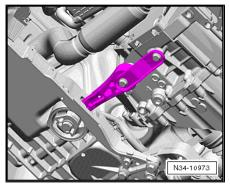
If fitted, remove the heat shield over the right-hand drive shaft. Tightening torque ⇒ Rep. Gr. 40; Repairing drive shafts
