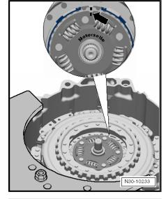
Turn clutch by hand and observe "small" engaging lever whilst turning.
