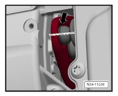
Plungers that are not seated correctly will damage mechatronic unit.
