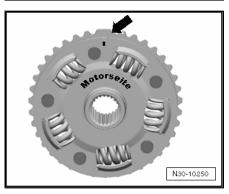
"Large" tooth has a mark on -engine end- -arrow-.
