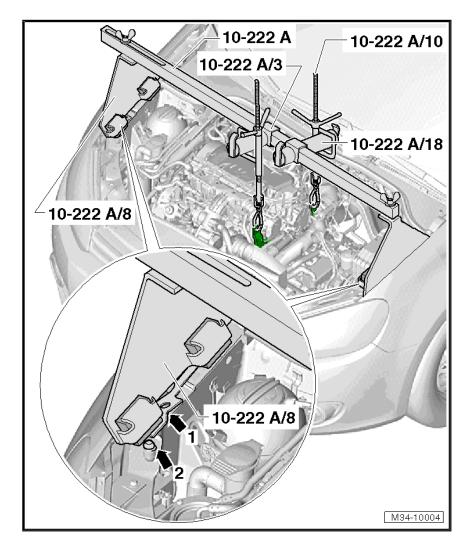
Place adapters -10 - 222 A /8- on upper longitudinal carriers, directly before the raised portion (-arrow 1-) next to bolt (-arrow 2-).
