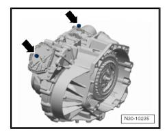
Turn gearbox with clutch upwards.
