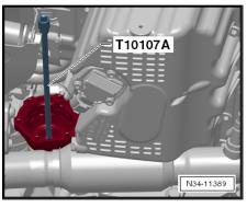
Remove all retainers and brackets from front of gearbox.
