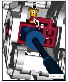
Attach cable with new locking plate on cable support bracket of selector mechanism.
