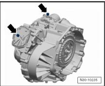
Secure gearbox on gearbox support -VW 353-
