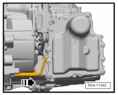
Unscrew bolts of mechatronic unit for dual clutch gearbox -J743- "in diagonal sequence".
