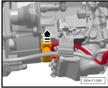
Pull cap off breather and close using a suitable plug to achieve an oil-tight seal.
