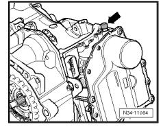
Remove all retainers and brackets from front of gearbox.
