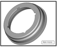
By "turning" bearing, check whether it is installed correctly and that grooves are seated correctly.
