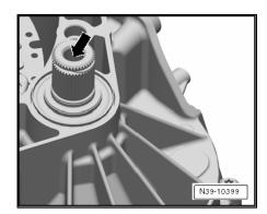
Half fill space between sealing lip and dust lip with sealing grease -G 052 128- -arrow-.
