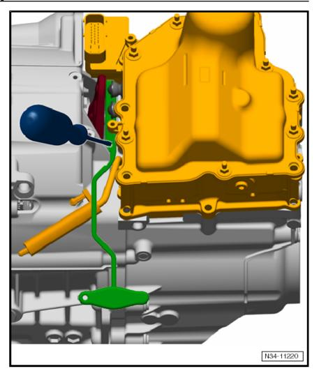
If lever slips off, this indicates you applied a bit of leverage to handle whilst turning.
