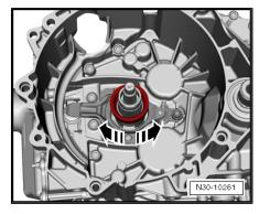
Place gauge block -T10374- on small bearing "with large opening upwards".
