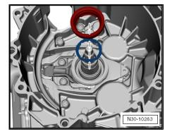
Small engagement bearing only fits in one position due to 4 grooves.
