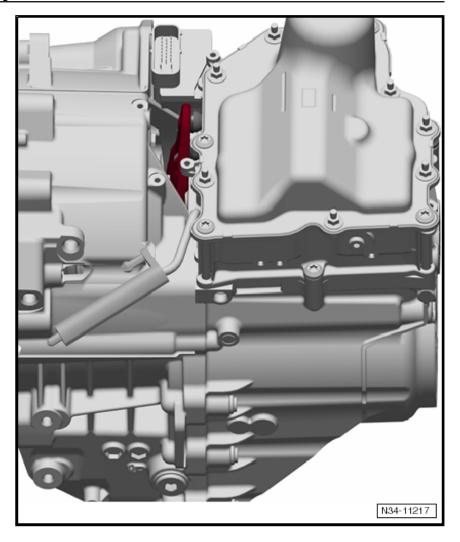
Insert assembly lever -T10407- to its right.
