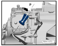
Install Bowden cable with loosened adjusting screw -arrowand new securing clip.
