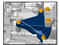
First bolt bracket to gearbox -1- with 40 Nm + 90° further turn.
