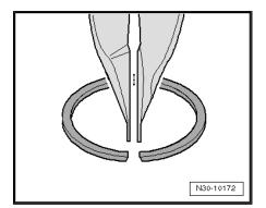
If you can insert retaining ring -arrow-, clutch is correctly pressed on to stop.
