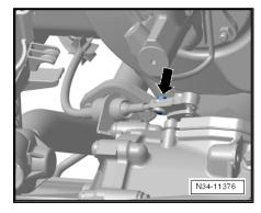
The gearbox lever must be pressed "completely to right side of vehicle" in the direction of selector lever cable support bracket.
