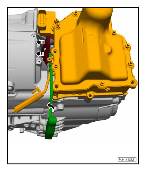
Do not take out assembly lever -T10407- . It must remain inserted between engaging lever and gearbox housing for the entire process.
