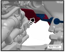
Loosen adjustment screw -arrow-.
