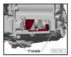
Make sure that all 4 gear actuators project 25 millimetres -a-.
