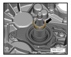
Place a ruler -T40100- on its side on flange of clutch housing. It should lie sideways on shaft end.
