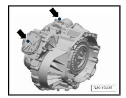
Securing clip for selector lever Bowden cable -arrow- must be renewed.
