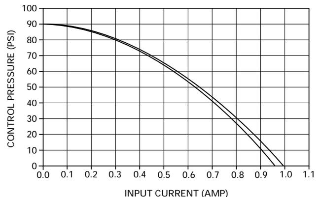
FIGURE C: PRESSURE CONTROL SOLENOID CURRENT FLOW
