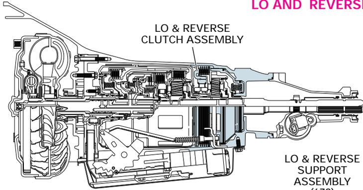
The lo and reverse clutch assembly is located in the rear of the transmission case and is applied in Park, Reverse and Manual First - First Gear. The steel clutch plates (682A,B,D) are splined to the transmission case while the fiber clutch plates (682C) are splined to the reaction planetary carrier (681). When applied, the lo and reverse clutch plates hold the reaction planetary carrier stationary to the transmission case.
