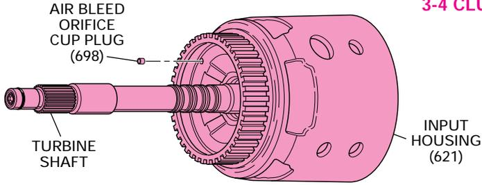
The 3-4 clutch assembly is located in the input housing and turbine shaft assembly (621) and is applied in Third and Fourth gears. The steel clutch plates (654B/C) are splined to the input housing while the fiber clutch plates (654A) are splined to the input internal gear (664). When applied, the 3-4 clutch plates transfer engine torque from the input housing to the input internal gear.
