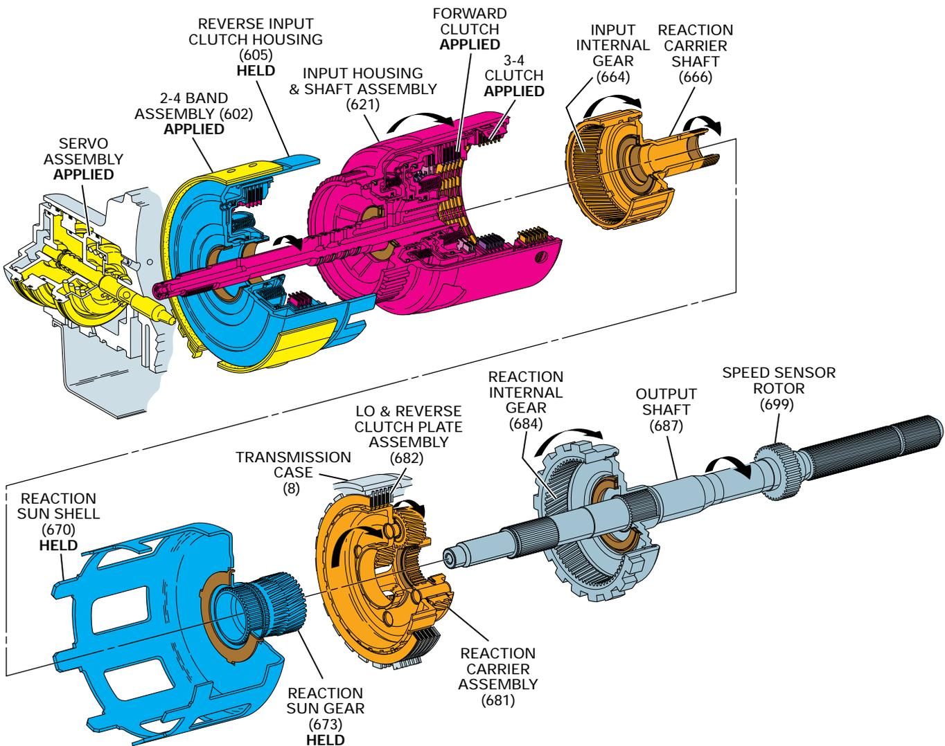
To maximize engine efficiency and fuel economy, an Overdrive gear ratio of approximately .73:1 is used. This allows the vehicle to maintain a given road speed with less engine output speed.
