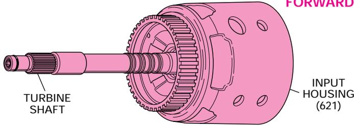
The forward clutch assembly is located in the input housing and turbine shaft assembly (621) and is applied in all forward drive ranges. The steel clutch plates (649A) are splined to the input housing while the fiber clutch plates (649B) are splined to the forward clutch outer race (644). When applied, the forward clutch plates transfer engine torque from the input housing to the forward clutch outer race and forward sprag clutch assembly.
