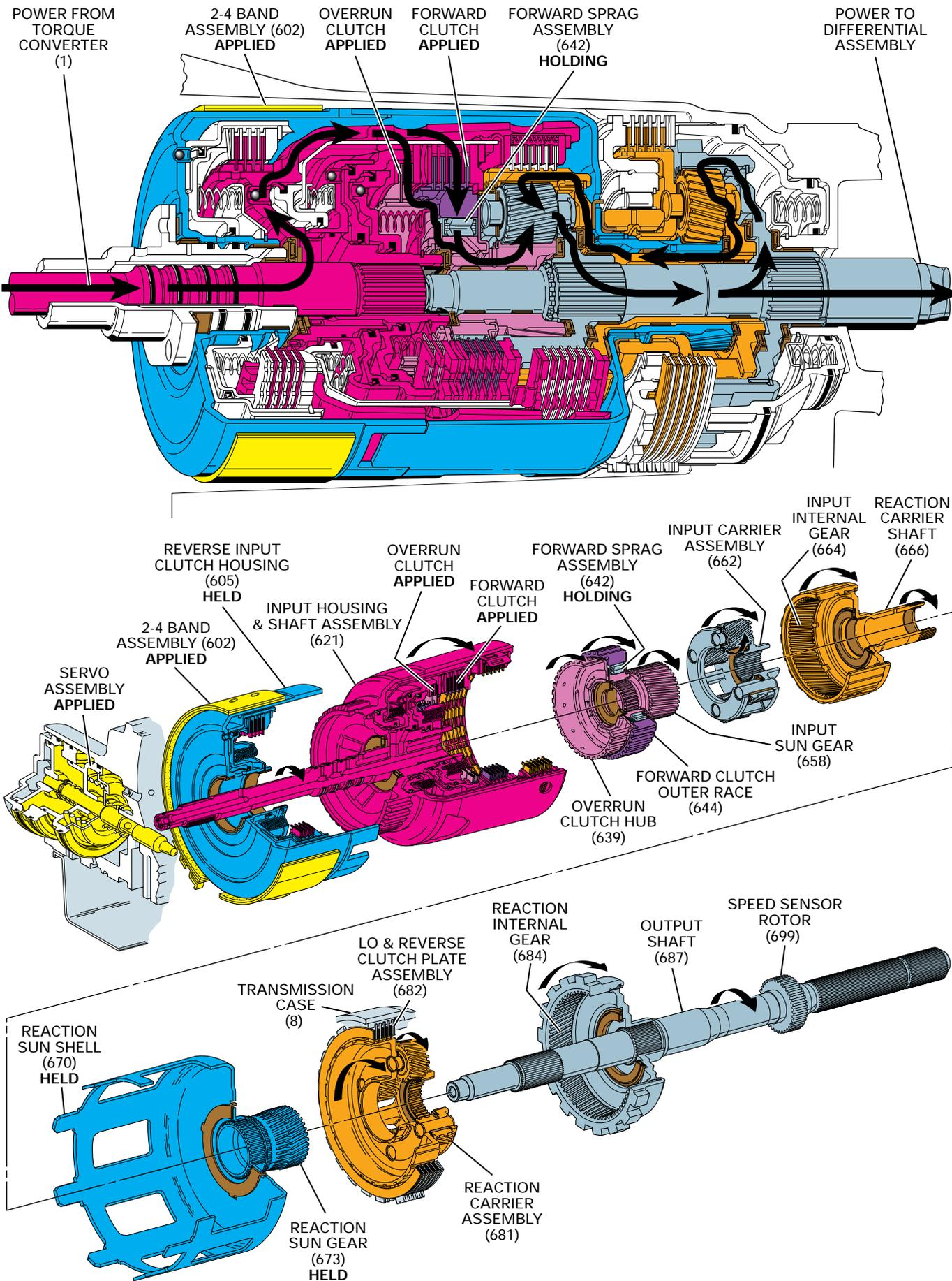
Manual Second gear range is available to the driver when vehicle operating conditions make it desirable to use only two gear ratios. These conditions include descending a steep grade when increased engine compression braking is needed, or to retain Second gear when ascending a steep grade for additional engine performance. The transmission immediately shifts into Second gear when Manual Second is selected regardless of vehicle speed (see Note below).
