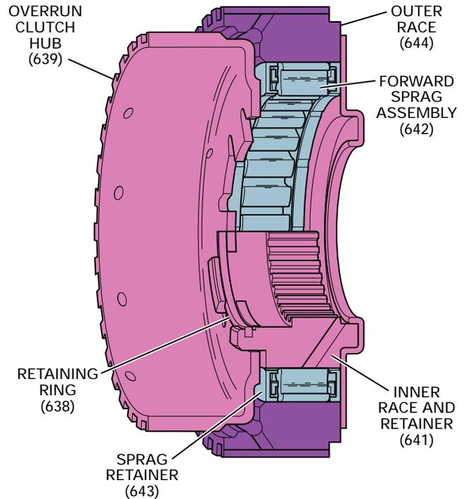
During coast conditions, power from vehicle speed drives the input sun gear faster than engine torque drives the forward clutch race (644). In this situation, the sprag race and retainer assembly (641), which is splined to the sun gear, overruns the sprag clutch and allows the vehicle to coast freely.
