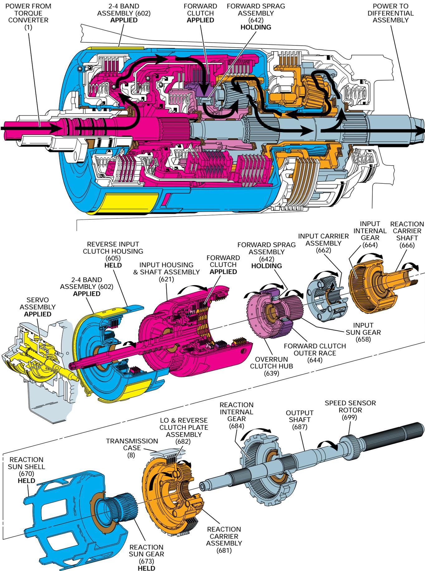
Input signals from the various engine and transmission information sensors are continually monitored by the Powertrain Control Module (PCM). As vehicle speed increases, the PCM processes this information to determine the precise moment to shift the transmission into Second gear. In Second gear, the planetary gear sets operate in reduction at a gear ratio of approximately 1.63:1.
