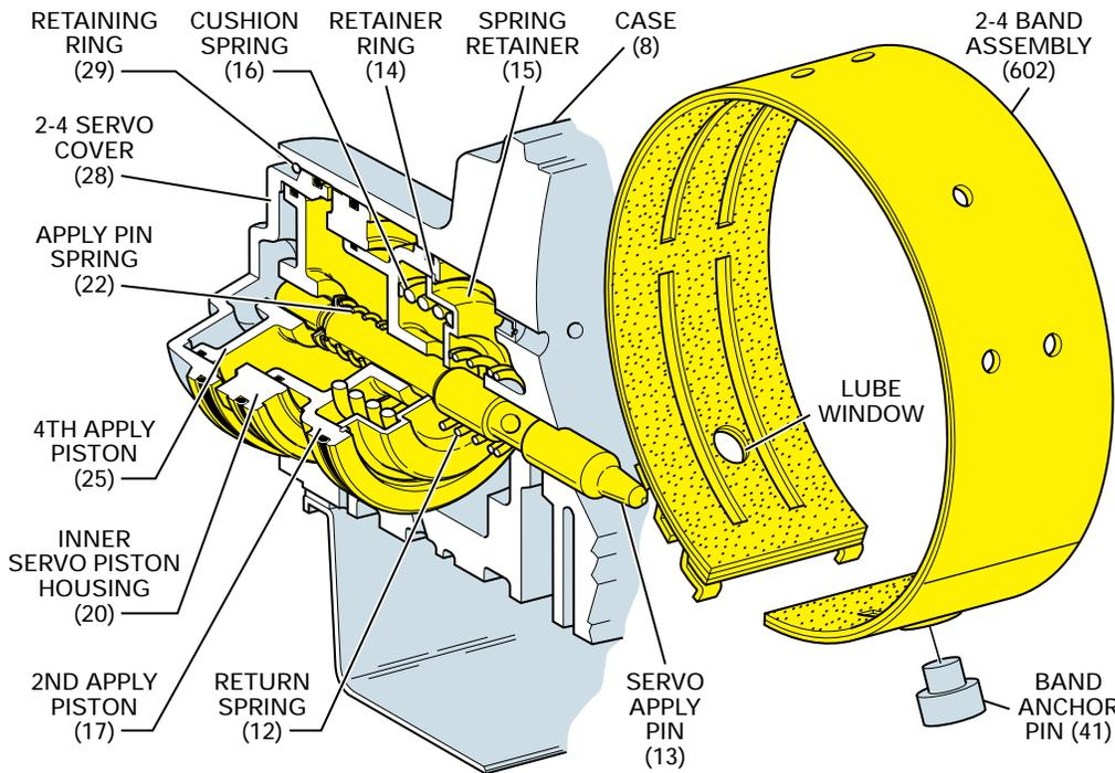
The servo assembly and 2-4 band (602) are located in the front of the transmission case and applied in Second and Fourth gears. In Third gear, the servo assembly releases the band and acts as an accumulator for the 3-4 clutch apply. The band is held stationary to the transmission case by the band anchor pin (49) and wraps around the reverse input housing (605). When compressed by the servo assembly, the 2-4 band holds the reverse input housing stationary to the transmission case.
