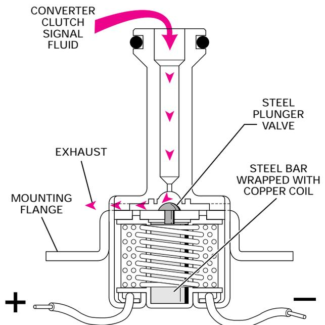
TORQUE CONVERTER CLUTCH SOLENOID (NORMALLY OPEN)
