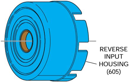
The reverse input clutch is located in the reverse input housing (605) and is used to provide an input to drive the vehicle in Reverse (R). The steel clutch plates (612A) are splined to the reverse input housing while the fiber clutch plates (612B) are splined to the input housing and turbine shaft assembly (621). When applied, the reverse input clutch transfers engine torque from the input housing to the reverse input housing.
