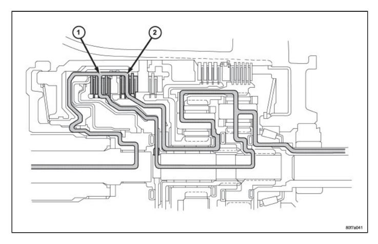
In third gear, two input clutches are applied to provide torque input: the underdrive clutch (1) and overdrive clutch (2). The underdrive clutch rotates the rear sun gear, while the overdrive clutch rotates the front carrier/rear annulus assembly. The result is two components (rear sun gear and rear annulus gear) rotating at the same speed and in the same direction. This effectively locks the entire planetary gearset together and is rotated as one unit. The gear ratio in third is 1:1.
