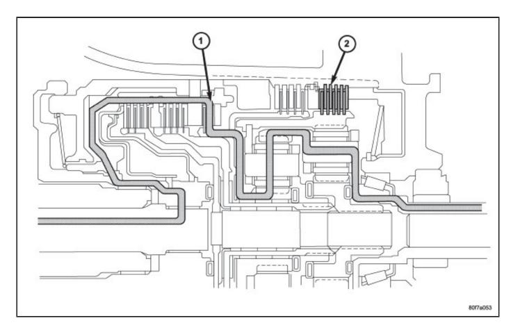
In reverse, input power is through the reverse clutch (1). When applied, the reverse clutch drives the front sun gear through the overdrive hub and shaft. The L/R clutch (2) is applied to hold the front carrier/rear annulus assembly stationary. The front carrier is being held by the L/R clutch so the pinions are forced to rotate the front annulus/rear carrier assembly in the reverse direction. Output torque is provided, in reverse, with a gear ratio of 2.21:1.
