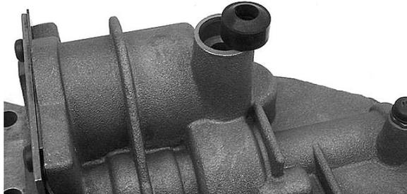
**Step 4:** Remove the 2-4 accumulator retainer bolts, and remove the plate and detent spring. Slide the accumulator and springs out of the valve body, and lay them aside.
