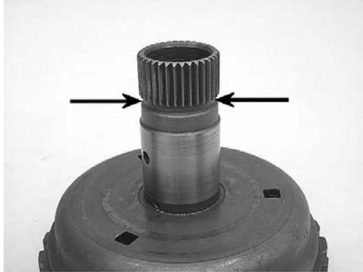
**Step 10:** Remove the tapered snap ring from the overdrive/underdrive reaction plate, being careful not to scratch the top of the reaction plate, which is a clutch apply surface.
