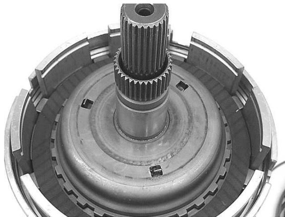
**Step 35:** Set the OD/reverse reaction plate into the input clutch drum, with the **Stepped** side facing down.
