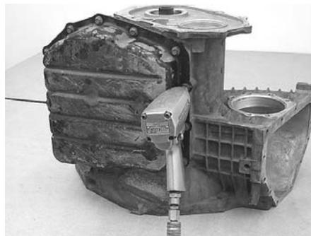
**WARNING:** Do not place the unit upside down, as this places the weight of the unit on the manual shaft. This can cause the valve body to almost explode off of the bottom of the case when the valve body bolts are almost all removed, ripping case threads and allowing the case to violently crash to the bench, possibly causing injury to the unit, the rebuilder, or both.
