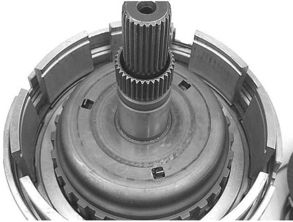
**Step 34:** Install the overdrive clutches into the input clutch drum.
