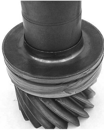
**Step 43:** Slide the transfer shaft into the case. You'll need an installer to push the race and baffle down into place. A two foot long piece of 1-1/2" ID plastic (PVC) pipe or something similar works well for this purpose.
