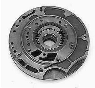
The 41TE uses a very straightforward, conventional crescent pump. There are no valve assemblies or intricate parts, other than screened checkball-controlled orifices in the stator support which are completely inaccessible.
