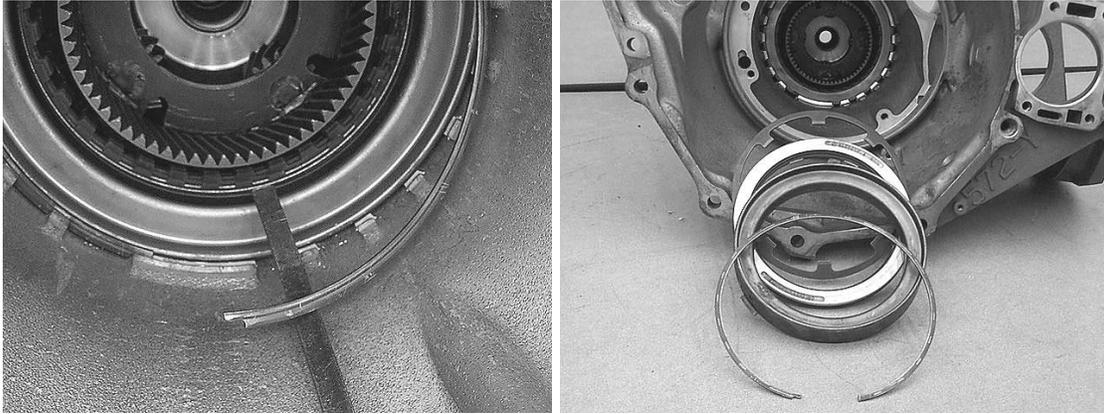
**Step 26:** Remove the 2-4 friction and steel plates from the case.
