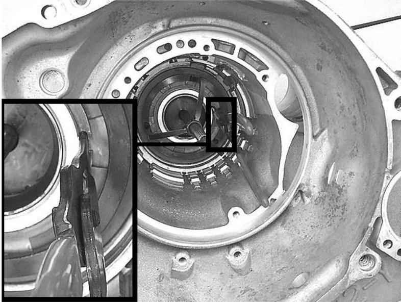
**Step 33:** Remove the low/reverse clutch return spring from the case.
