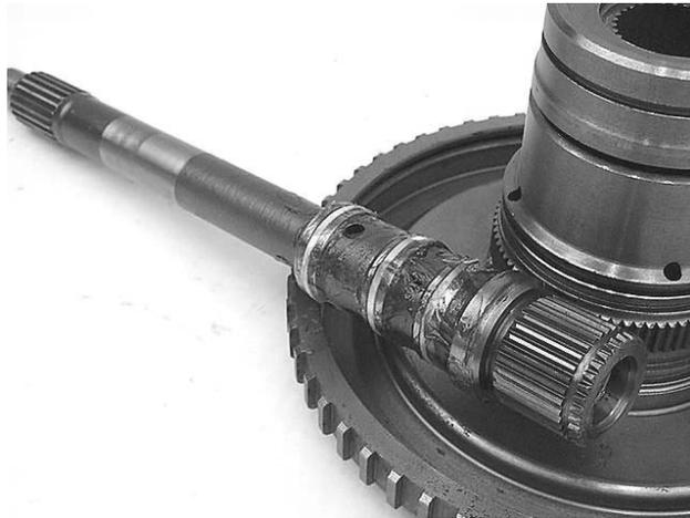
**Step 3:** Use a suitable press to press the input shaft into the input shaft hub.
