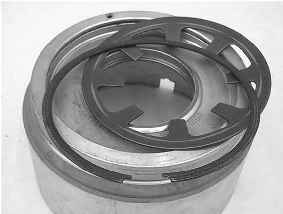
**Step 22:** Remove the lip seal from the groove inside the input drum.
