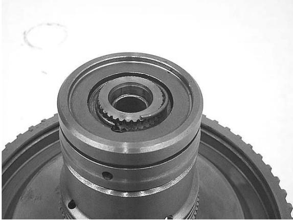
**Step 5:** Install the two lip seals and two o-rings onto the input hub.
