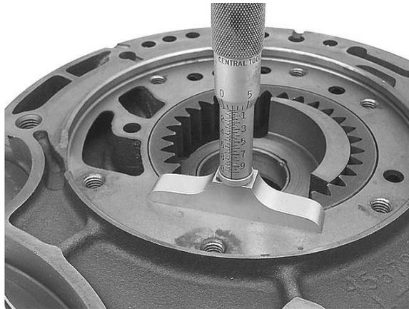
Clearance between the top of the inner pump gear and the top of the pump pocket should be less than 0.002".
