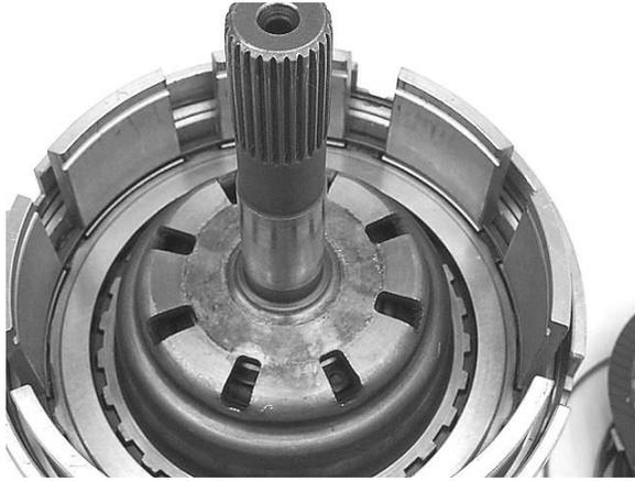
**Step 31:** Install the #3 thrust washer (5 locating tabs) on the underdrive shaft hub. Use assembly lube to hold the washer in place.
