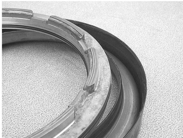
**Step 19:** Install the 2-4 clutch piston and housing in the case, making sure that the return spring tabs line up with the notches in the 2-4 piston. The piston housing has a tab that must be lined up with a slot in the bottom of the case to ensure that the apply oil port in the housing lines up properly with the apply passage in the valve body.
