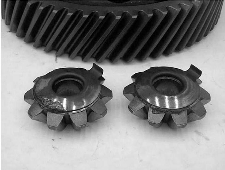
**NOTE-** the pinion gear washer tangs can only enter the differential carrier from one side, through the slots that lead to the pinion shaft holes. Make sure you slide the pinion gear tangs through these slots.
