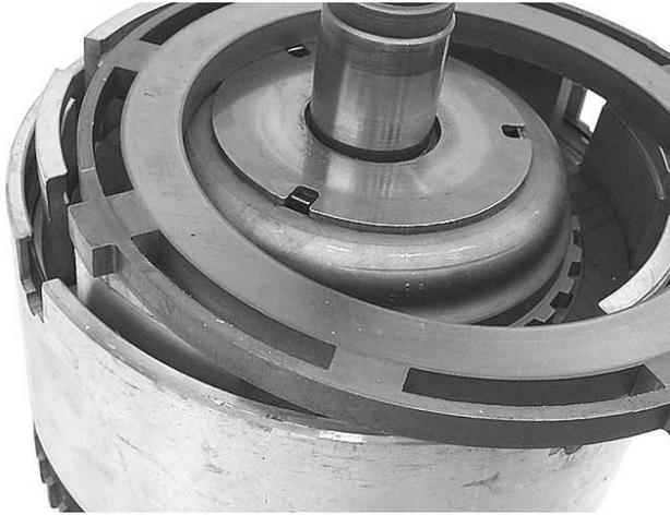
**Step 7:** Remove the waved lower OD/reverse clutch snap ring from the input clutch assembly.
