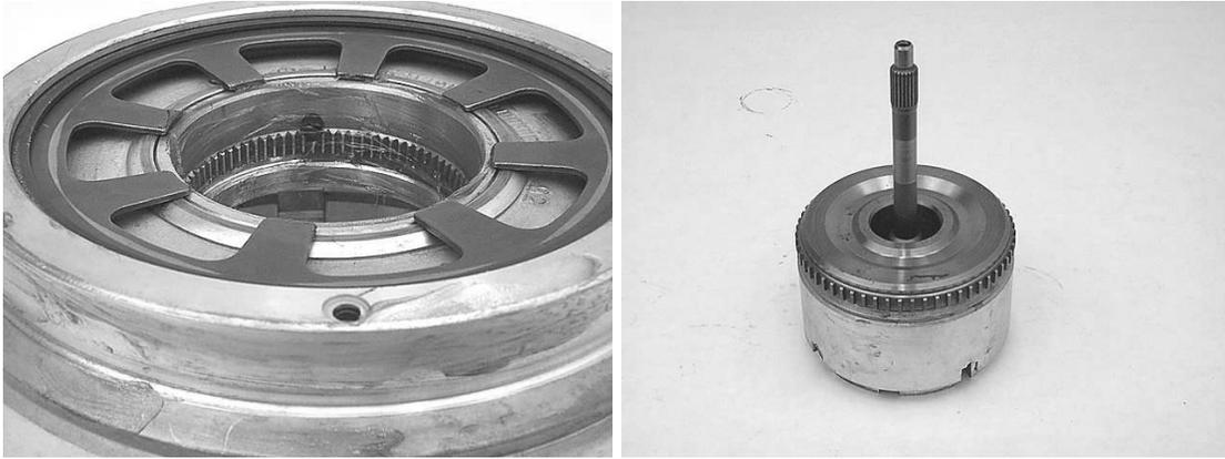
**Step 11:** Flip the assembly, and install the retaining snap ring onto the hub, with the tapered side of the snap ring facing up. Use a screwdriver and hammer to gently set the snap ring all the way into the groove. When seated, the gap between the ring ends is approx. 1/4".
