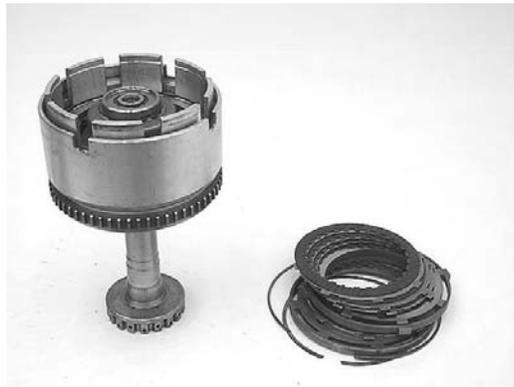
**Step 29:** Install the #2 thrust bearing on the input hub. Use assembly lube to hold the bearing in place.
