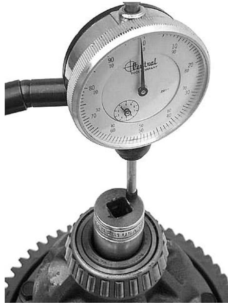
Side gear endplay should be between 0.001" and 0.013" (0.02 mm to 0.35 mm). Replace the selective side gear thrust washers to adjust the endplay.
