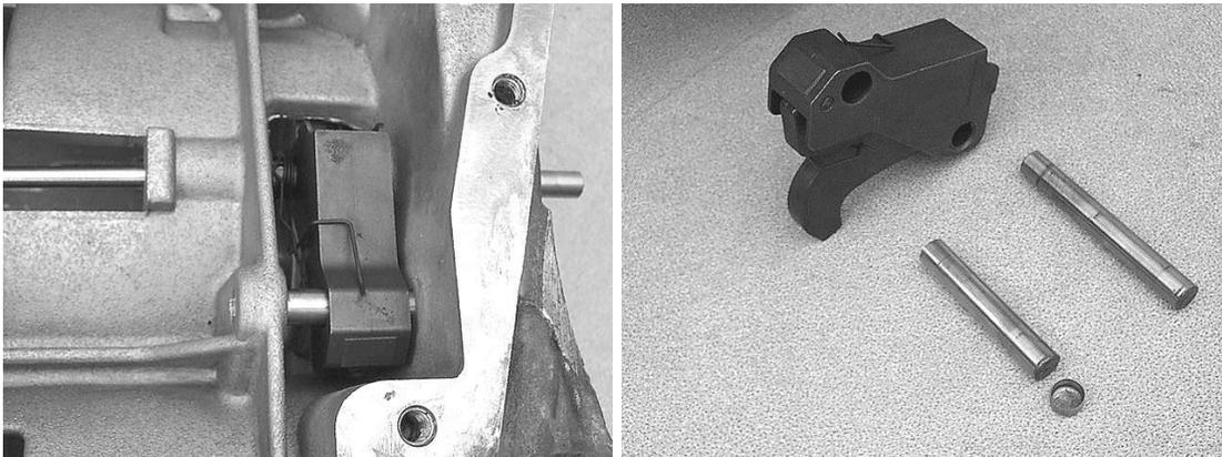
Removing the park pawl and **stamped steel** guide (guide has only one pin hole): Using a long thin screwdriver or punch, tap the park pawl guide pivot pin out, and remove the park pawl and guide bracket from the case. If it seems stuck, slowly rotate the rear planetary carrier while pulling on the bracket.
