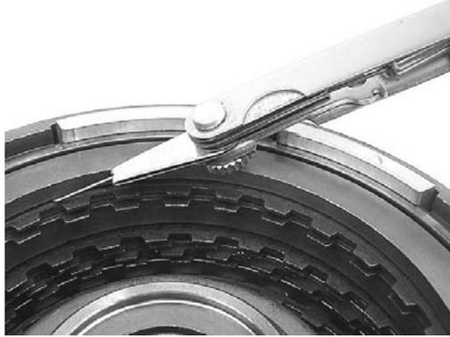
**Step 28:** Remove the overdrive and reverse clutches from the clutch drum, and lay them aside for installation later. Make sure you keep these clutch stacks separate, so you don't mix them up later.
