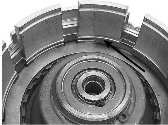
**Step 17:** Install the last thin friction plate in the underdrive stack, and then lay the reaction plate in place. Be sure the reaction plate is oriented correctly, because it can get confusing- If the plate has only one **Step**, this **Step** goes down. If it has two **Steps**, the **Step** at the lug goes down and the **Step** partway across the apply surface goes up.
