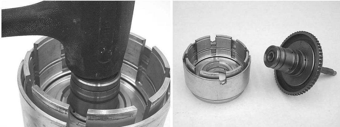
**Step 19:** Pull the input clutch retainer out of the OD/reverse piston. Remove the lip seal from the groove inside the OD piston. Remove the o-ring from the groove in the inside diameter of the piston.
