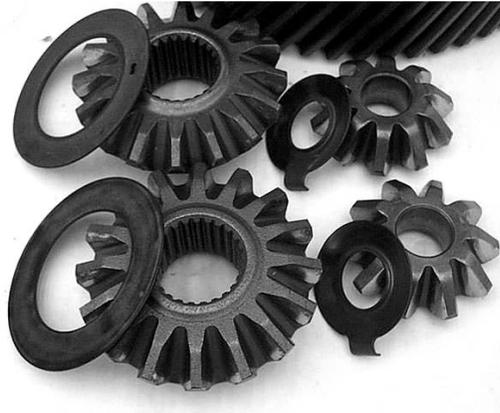
**Step 6:** Check the gears, pinion shaft and thrust washers for wear or damage.
