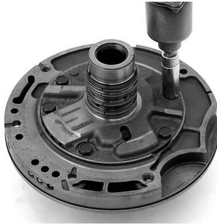
**Step 4.** Remove the pump gears from the pump body pocket.
