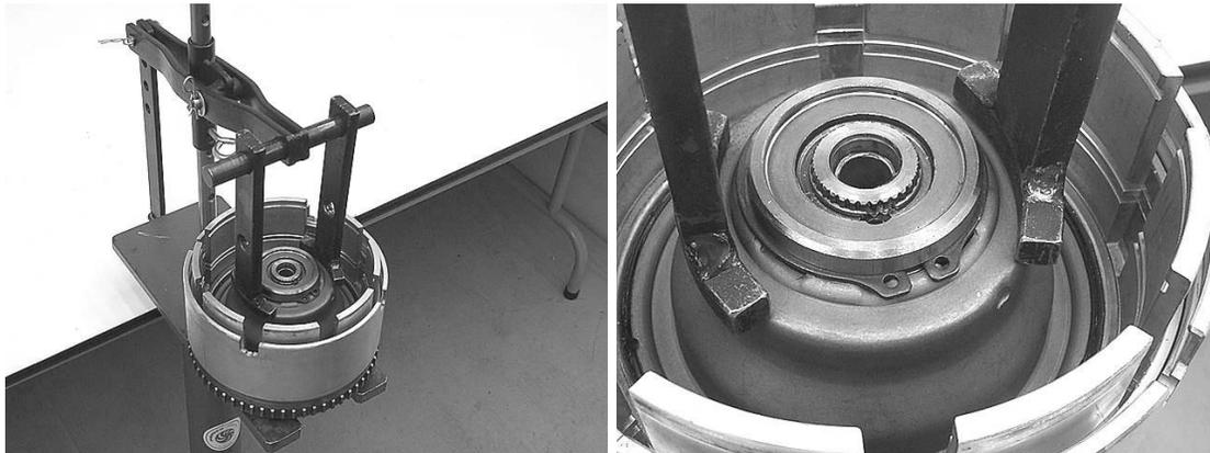
**Step 15:** Install the underdrive clutch stack in the clutch drum; leave out the top friction plate for now. This will include four thin steel plates and three thin friction plates.
