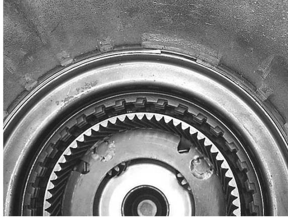
**NOTE-** Some technicians choose to use a hammer and large screwdriver to install the snap ring without the aid of any compressor tool. This can be successful and easy, but be sure to install both snap ring ends in the top case lug, and be sure to tap the snap ring all the way into the ring groove in the case.
