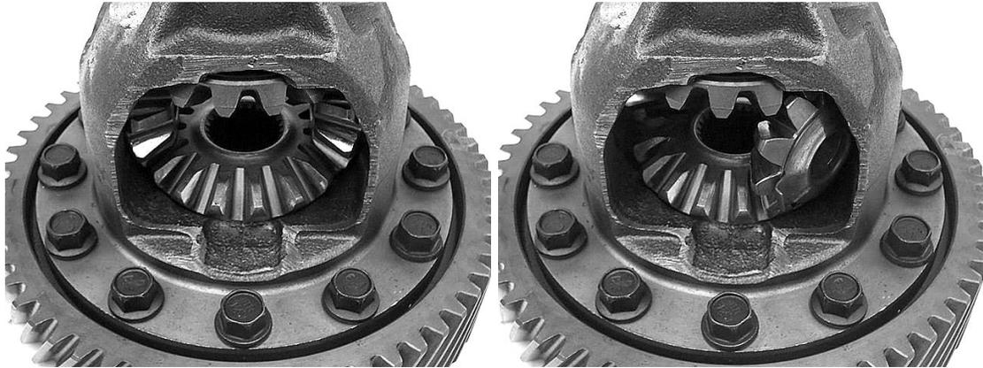
**Step 5:** Remove the side gears from the housing.
