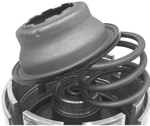
**Step 16:** Remove the underdrive piston from the drum. Check the inside diameter for wear from the input hub where the lip seal rides.
