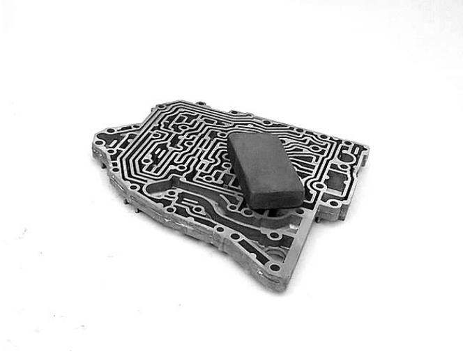
**Step 9:** Resurface the 2-4 accumulator bore. A brake hone is good for this, but be sure not to remove too much material from the bore, just enough to clean up the surface. Smooth the texture a bit with some Scotch-Brite™.
