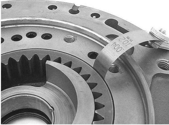
Clearance between the top of the outer pump gear and the top of the pump pocket should be less than 0.002".
