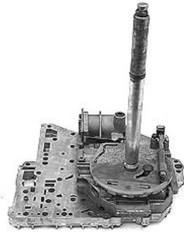
**Step 1:** Remove the retaining screw from the rooster comb, and lift the manual shaft off of the valve body.
