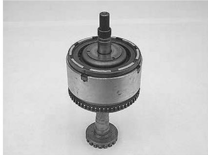
NOTE- The stand being used to support the drum is not a 41TE part. This is a 4T60 (440T4) 4<sup>th</sup> clutch shaft and hub.
